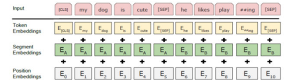
Figure 2: BERT input representation. The input embeddings are the sum of the token embeddings, the segmentation embeddings and the position embeddings.
